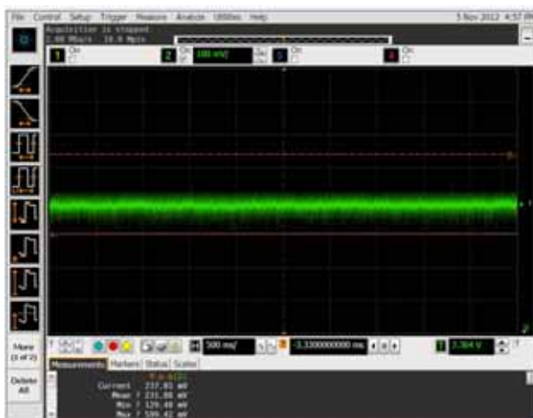
Fig. 1.4. Output noise of amplifiers when PRT at input
