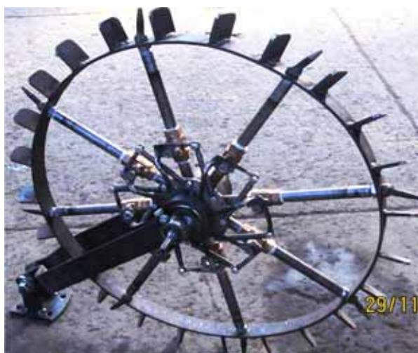
Fig. 1. View of developed nitrogen (liquid urea) metering mechanism
