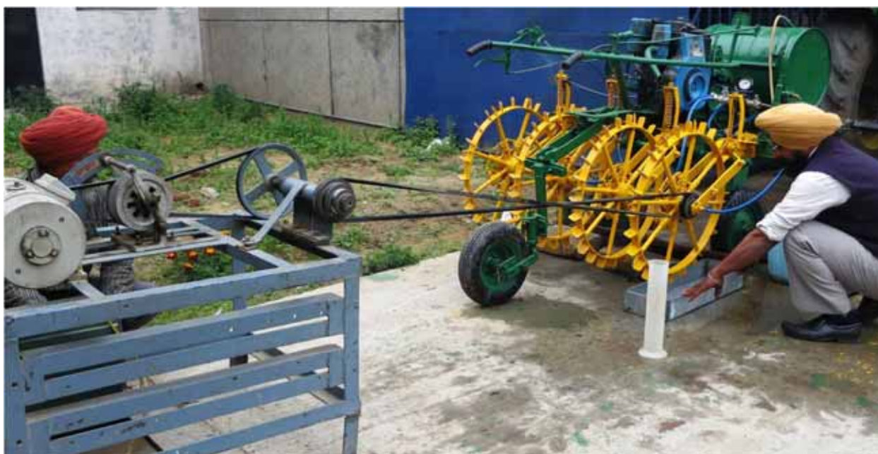
Fig. 2. View of the laboratory evaluation of nitrogen (liquid urea) metering mechanism
